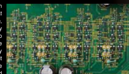
A fully balanced circuit from the D/A converter to the XLR OUT terminals
